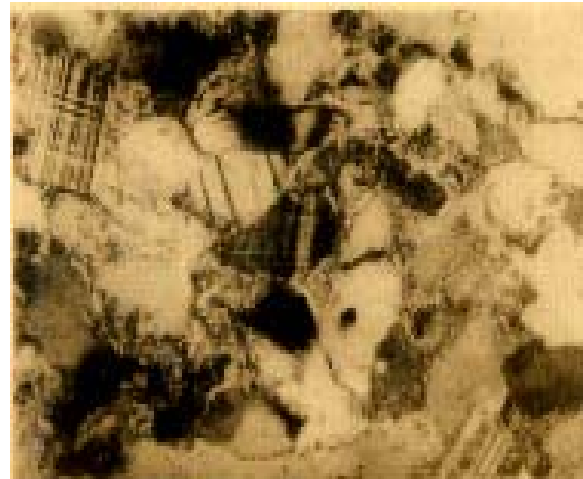
Figure 2: Photograph of a Sample of Amenu Sandstone, Taken Under Crossed Polars, Showing Abundance of Quartz and Feldspar. Magnification X28.
