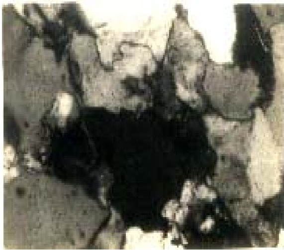
Figure 7: Photograph of a Sample of Akpoha Sandstone, Taken Under Crossed Polars, Showing Poor Sorting and Sub-Angular to Sub-Rounded Shape of the Rock. Magnification X25.
