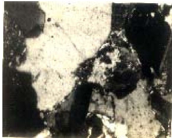
Figure 5: Photograph of a Sample of Amenu Sandstone, Taken Under Crossed Polars, Showing Crushing of Quartz Grains at Inter-Grain Boundaries. Magnification X25.
