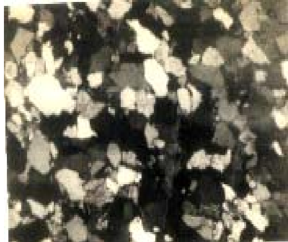
Figure 8: Photograph of a Sample of Ibii Sandstone, Taken Under Crossed Polars, Showing the Fine Grained Nature of the Sandstone. Magnification X32.
