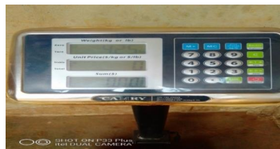
Plate 5: Scale used to Measure the Initial and Final Measurement of the Gas Cylinder.
