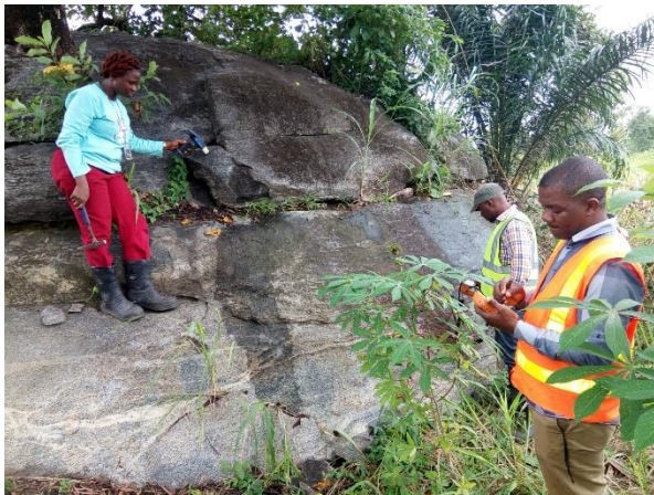
Figure. 2: The hand-held GDD Magnetic Susceptibility Meter is small and easy to use. Measurements are taken first on the rock surface followed by reference reading with another meter.
