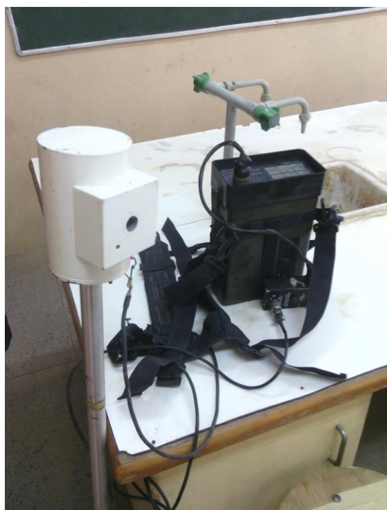
Plate I: Shows the G-856-Mag TM Proton Precision Magnetometer used for the Magnetic Data Acquisition.
