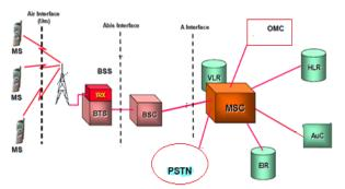
Figure 2: GSM Architecture (how different network elements form a GSM network).
