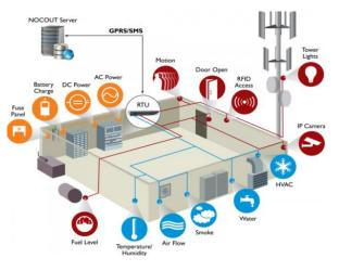
Figure 3: BTS (has different parts that are working together as a cell).
