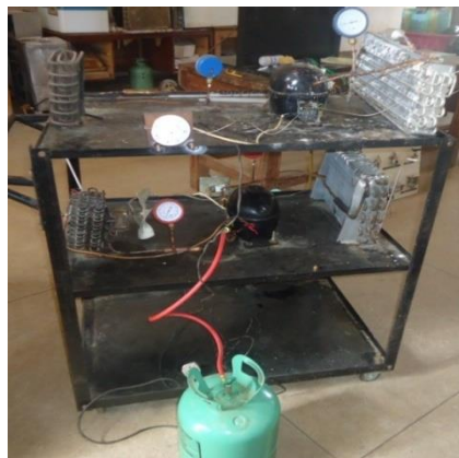
Figure 1: A Typical Setup for Investigating the Coefficient of Performance of the Refrigerants.
